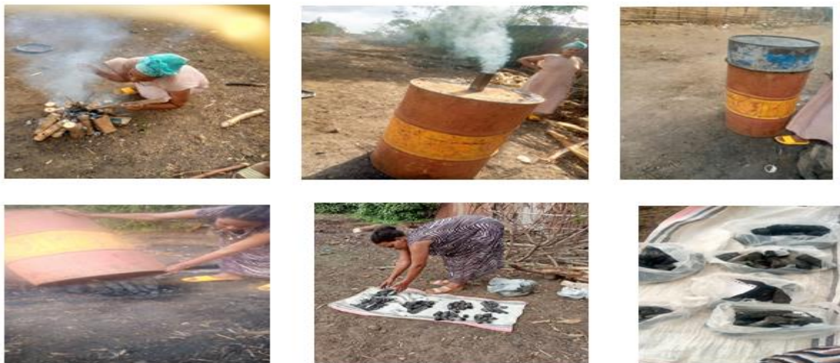
figuer 3. 3. Carbonization and charcoal production from Acacia brevispica
