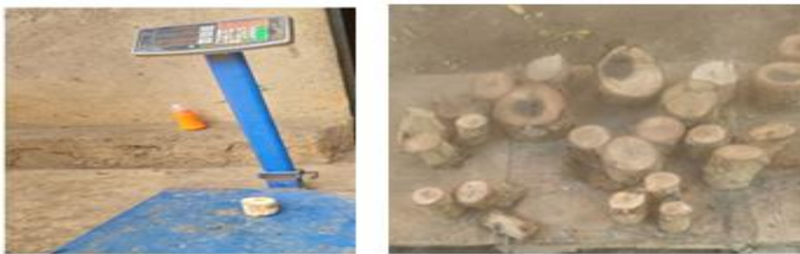
figure 3. 4. Air drying the sample and measuring the weight of specimens
