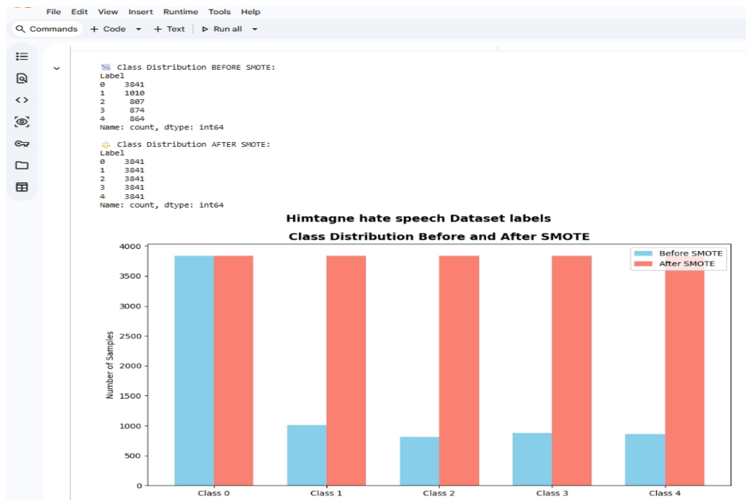
Figure 44 Classes Distribution Before and After SMOTE Graph
