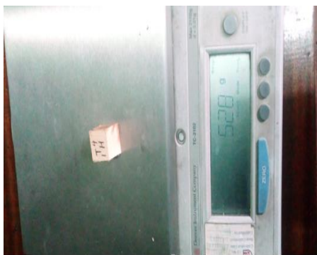
Figure 6: The weight of the specimens sampled was measured on a digital balance.
