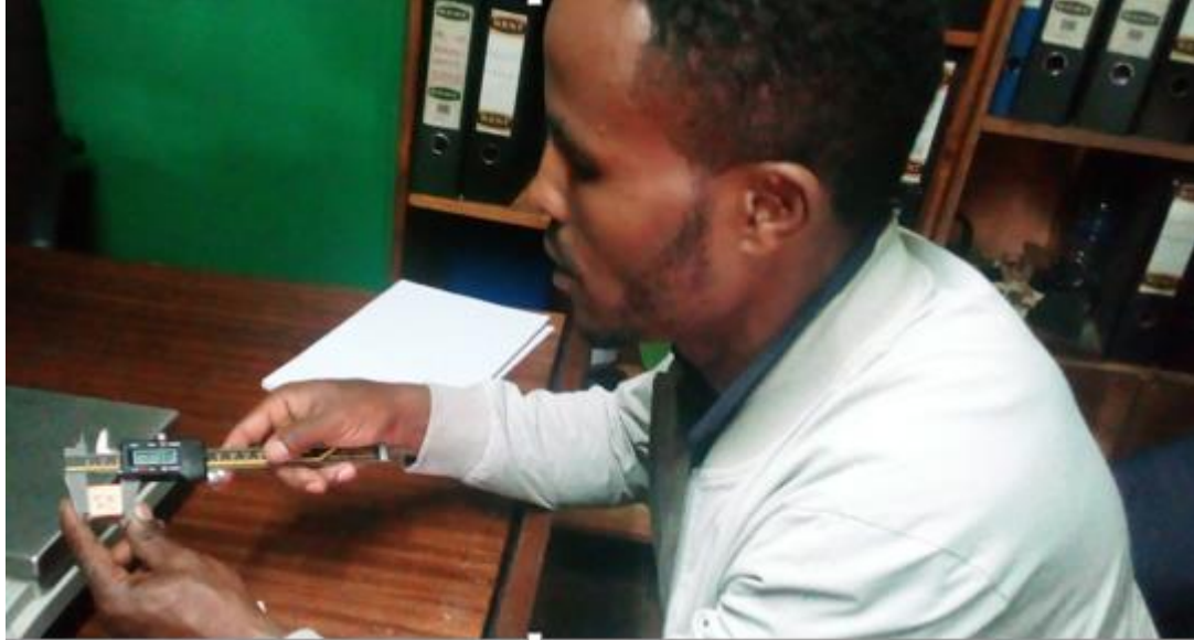
Figure 8: The first dimensions of the specimen were measured (using a digital Vernier caliper) in green condition in the three anatomical directions (radial, tangential, and longitudinal).
