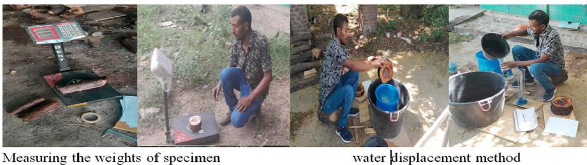
Figure 5 The process of measuring the density through water displacement methods
