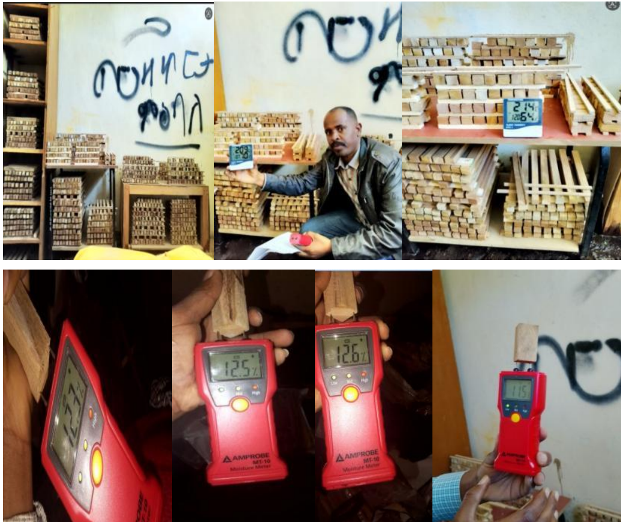
Figure 3.6. Drying green specimens to 12% MC for mechanical testing
