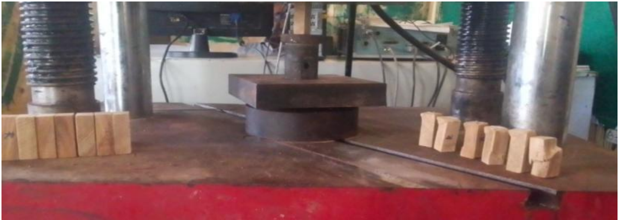
(a), Testing setup before & after load application.
