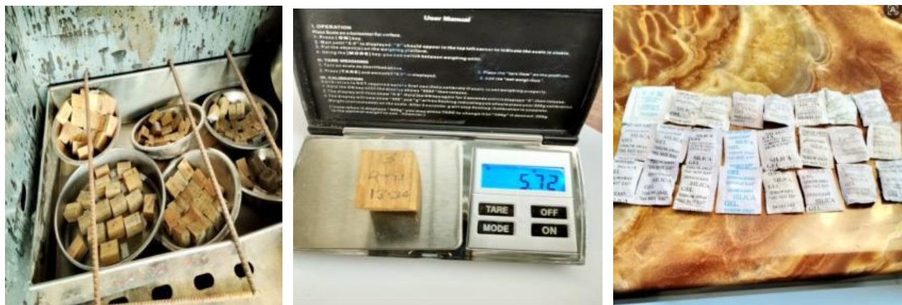
Figure 3.9. Basic density determination by measuring oven-dry mass and controlling moisture absorption with silica Gel.
