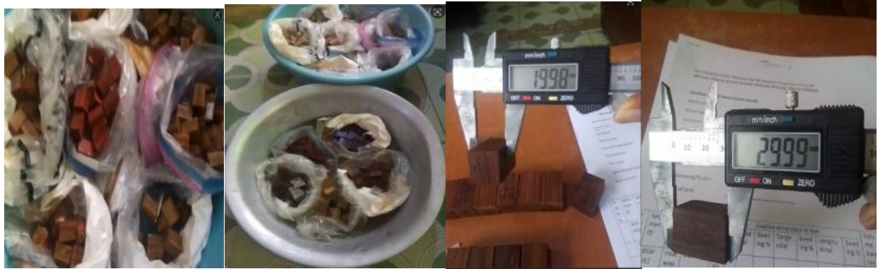
Figure 3.11. Cordia africana specimens swelling test procedure & measuring swollen dimensions
