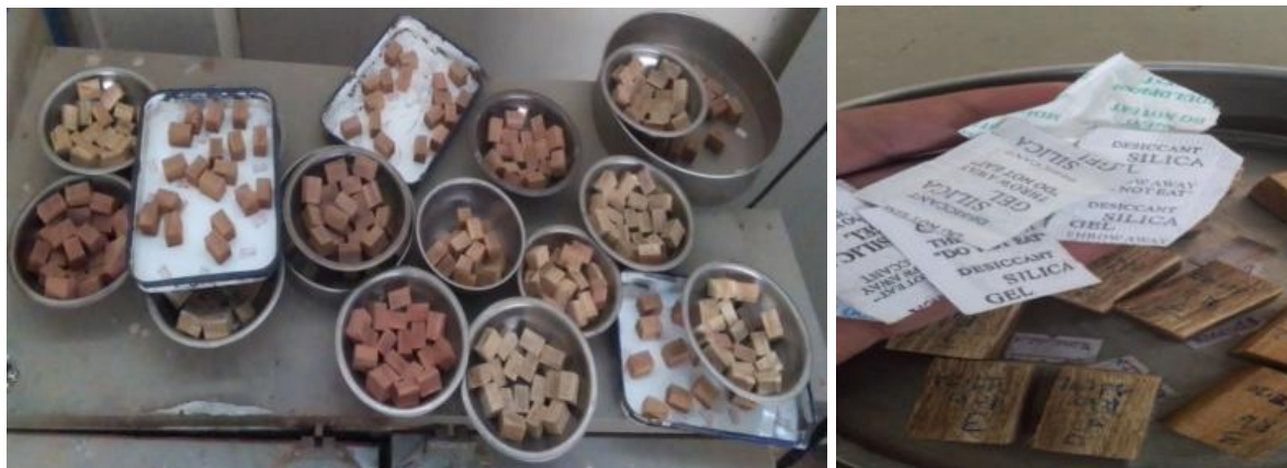
Figure 3.8. Measuring moisture content green to oven-dry using oven-dry and controlling moisture absorption using silica Gel
