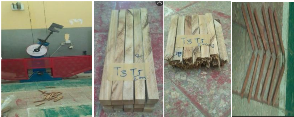
(a), Charpy pendulum hammer (b), Tested SW specimens (c), Tested HW specimens
