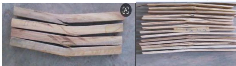
(C), Static bending strength tested sapwood specimens
