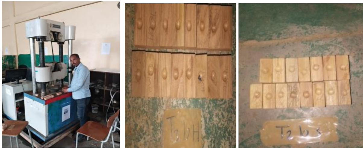
(a), UTM (b), Hardness tested HW specimens (c), Hardness tested SW specimens
