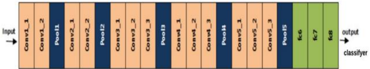
Figure 2.18 The Architecture of VGGNet [49]
