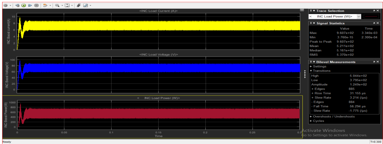
Figure 5.22.PV module output power voltage and current with INC method under PSC and the TCT connecting scheme Using the DC-DC boost converter
