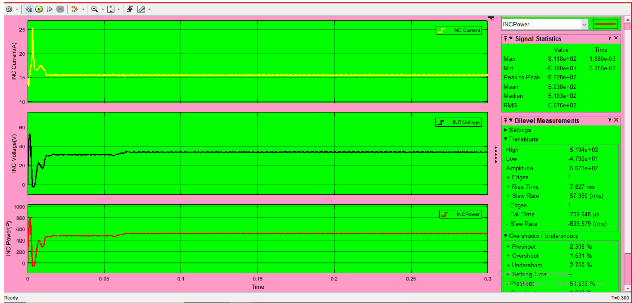
Figure 5.24. output power Voltage and Current of PV Module in INC Method under partial shade condition and BL interconnection scheme before boost of DC-DC converter
