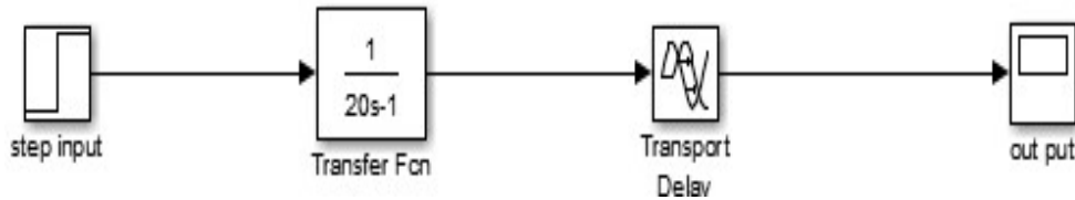
Figure:5.1 TDUP Open-loop Step Response Simulink diagram(Example1)
