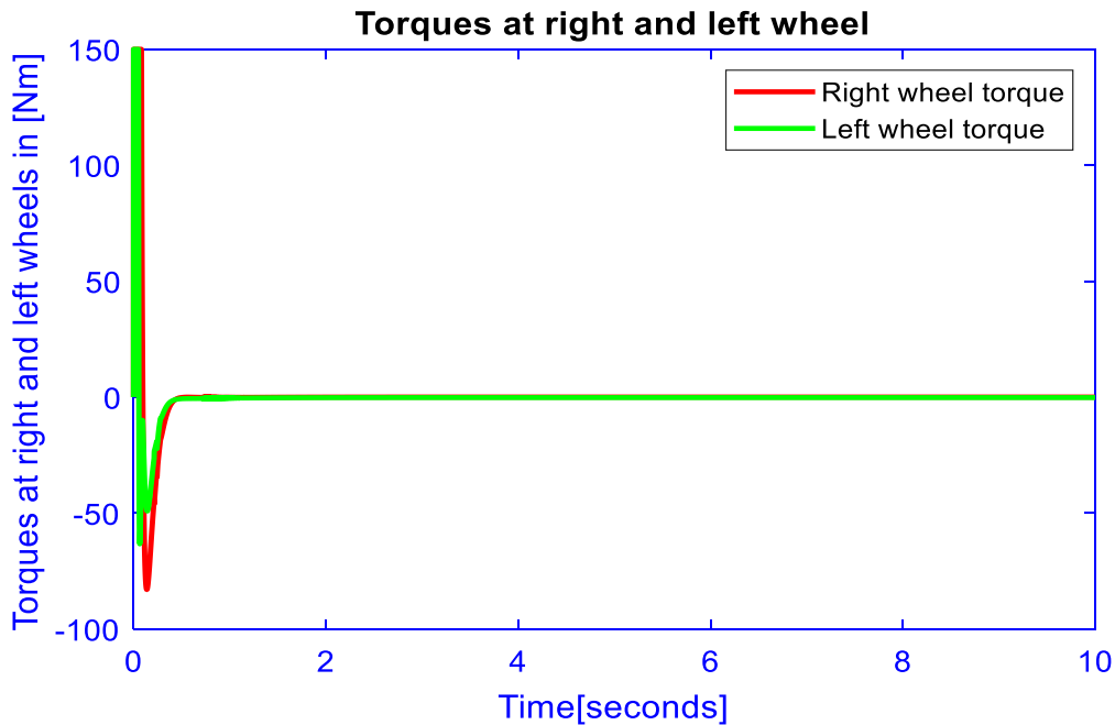
Figure 5.13: Torque control input for right and Left motor.
